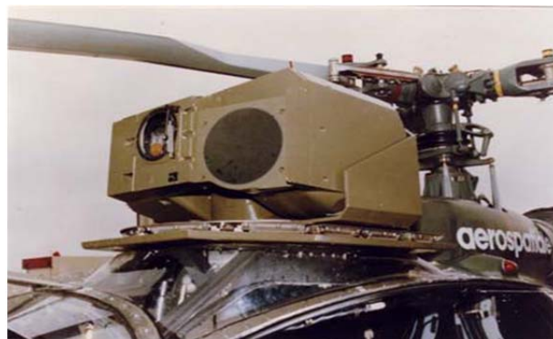
Fig. 3: THE OPTO-ELECTRONIC SYSTEM MOUNTED ON A HELICOPTER REQUIRES VIBRATION ISOLATION.
